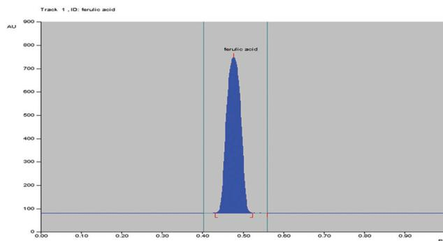
Figure 1: Chromatogram of standard ferulic acid.
