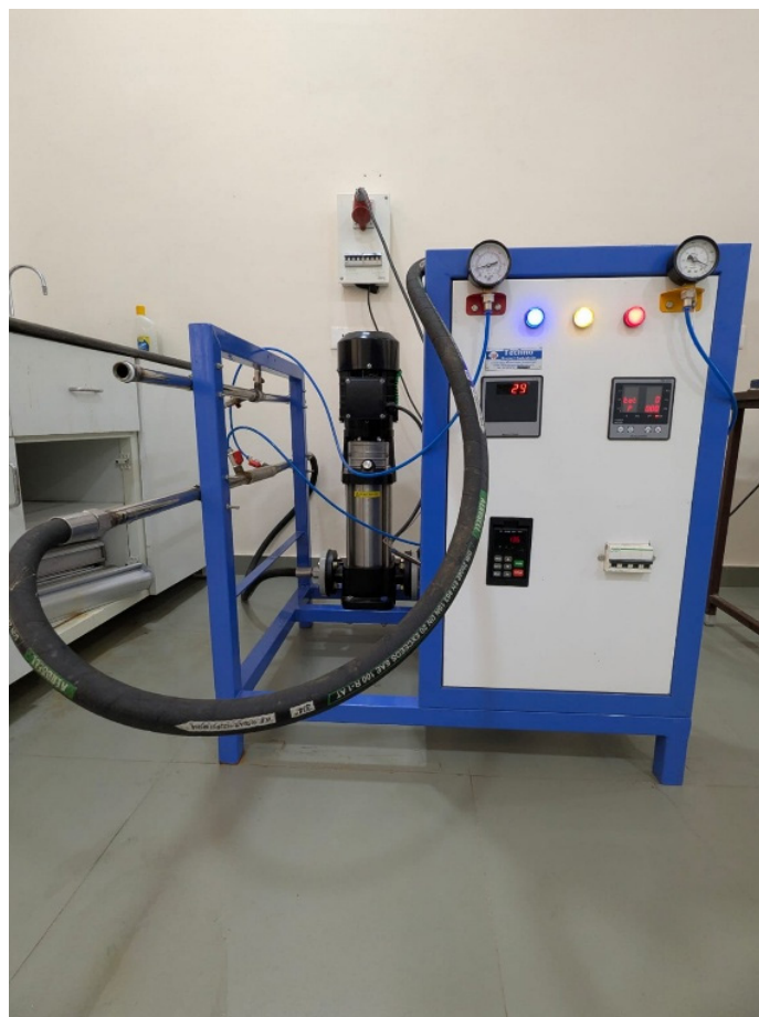
Figure 1: Experimental setup for hydrodynamic cavitation.
