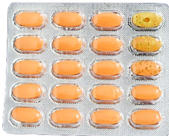
Figure 2(b): Defective Film-coated tablet.
