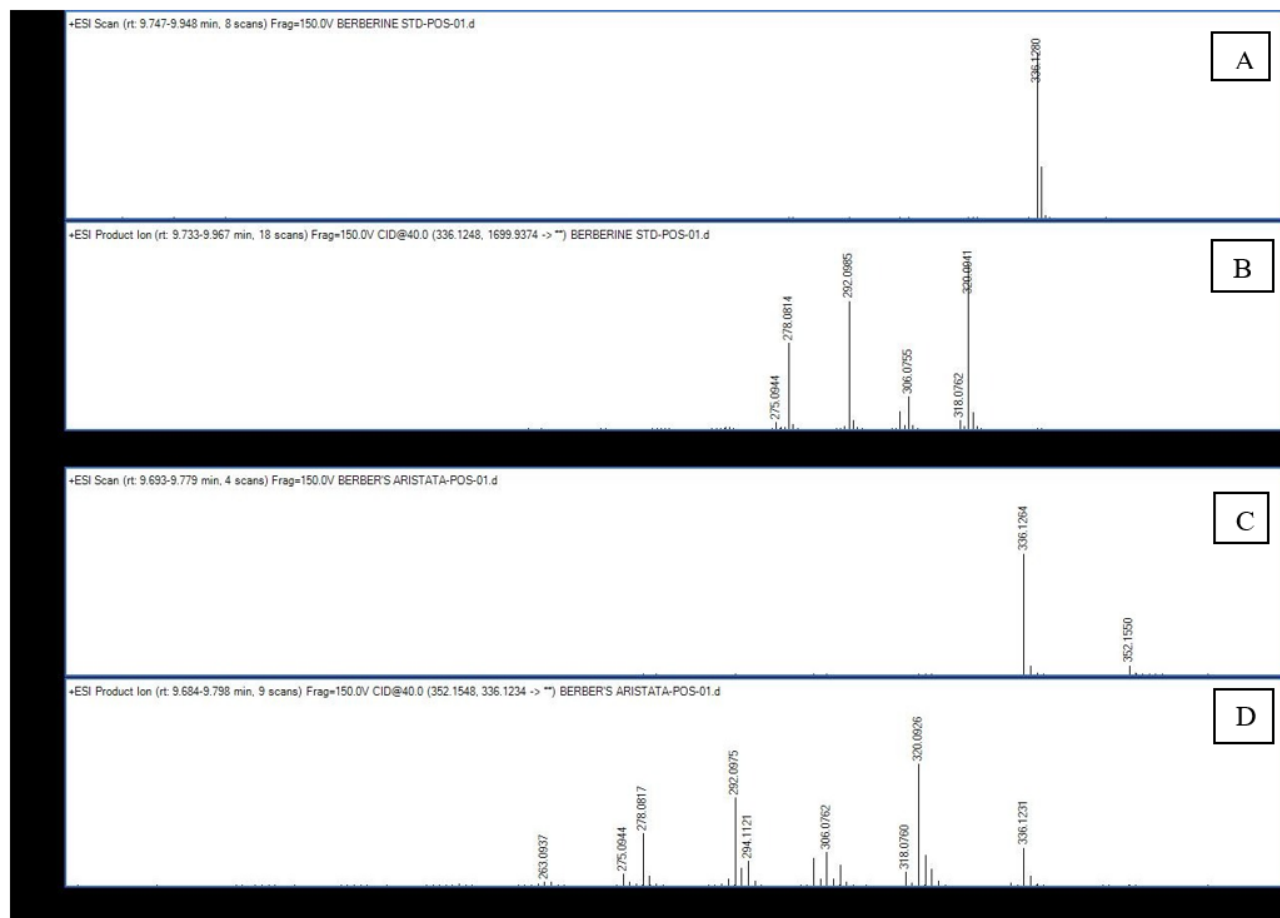
Figure 2: a) LC-MS spectra of standard berberine. b) LC-MS/MS spectra of standard berberine. c) LC-MS spectra of isolated berberine. d) LC-MS/MS spectra of isolated berberine.
