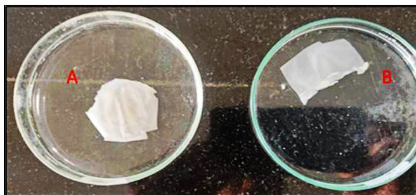
HET-CAM Test (A) Treated with 0.9% NaCl (B) Treated with the F6 Emulgel
