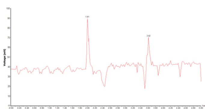
Figure 2: Chromatogram Obtained from (Methanol: Acetonitrile (a) 70:30 v/v and (b) 50:50) Mobile Phase with Zorbax C8 (100×4.6 mM, 5 μM) column.
