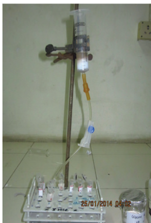
Figure 10: It shows the partial purification of alkaline protease by gel filtration chromatography using Sephadex G-75
