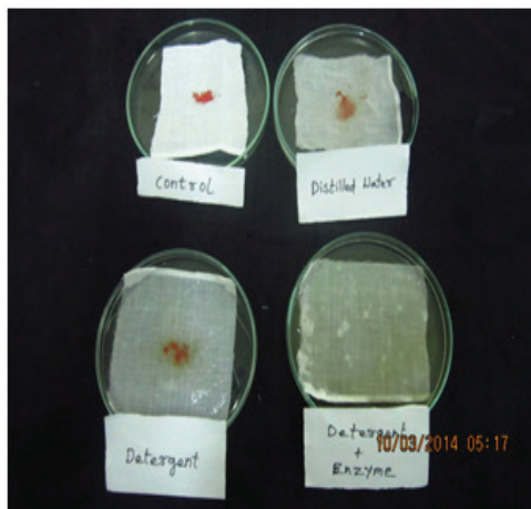
Figure 13A: It shows the de-staining activity of the detergent with enzyme (alkaline protease) additive on blood stains
